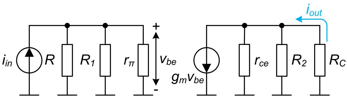
$$i_{in} = \left( \frac{1}{R_1} + \frac{1}{R} + \frac{1}{r_\pi} \right) v_{be}$$
