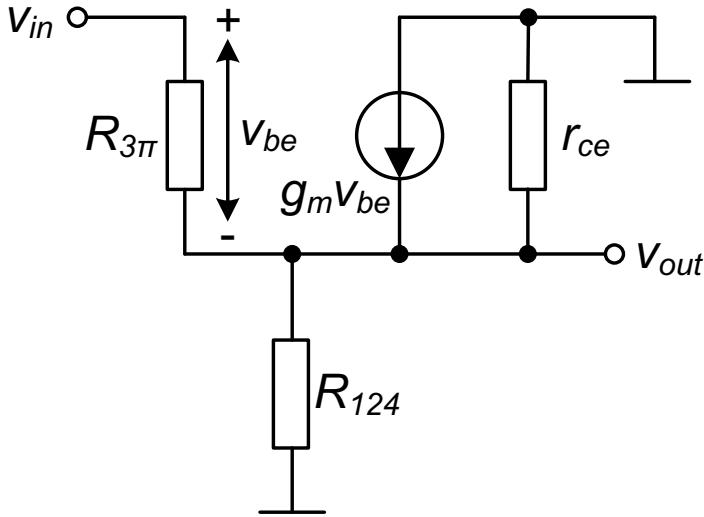
$$R_{3\pi} = R_3 \parallel r_\pi = 660.7 \Omega$$
