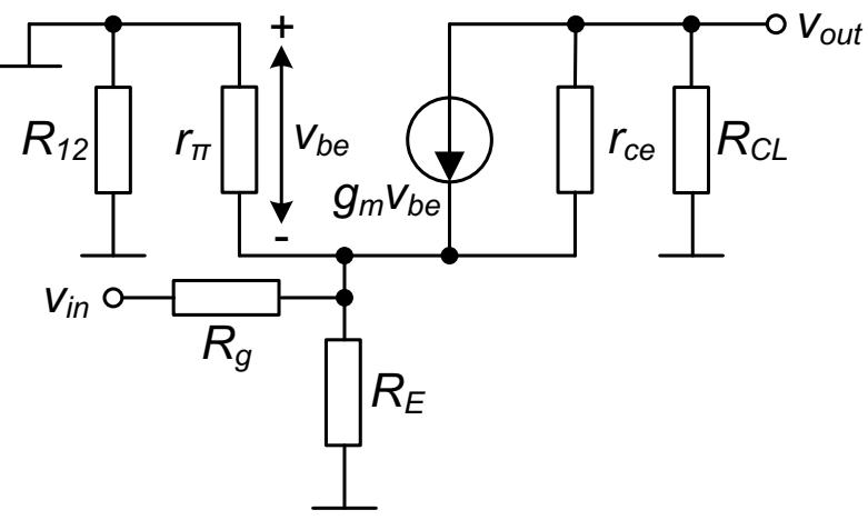
$$\frac{v_{be}}{r_\pi} + g_m v_{be} + \frac{v_{in} + v_{be}}{R_g} + \frac{v_{be}}{R_E} = 0$$
