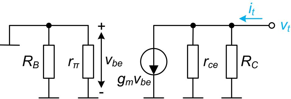
$$R_{out} = \frac{v_t}{i_t} = R_C = 2 \text{ k}\Omega$$
