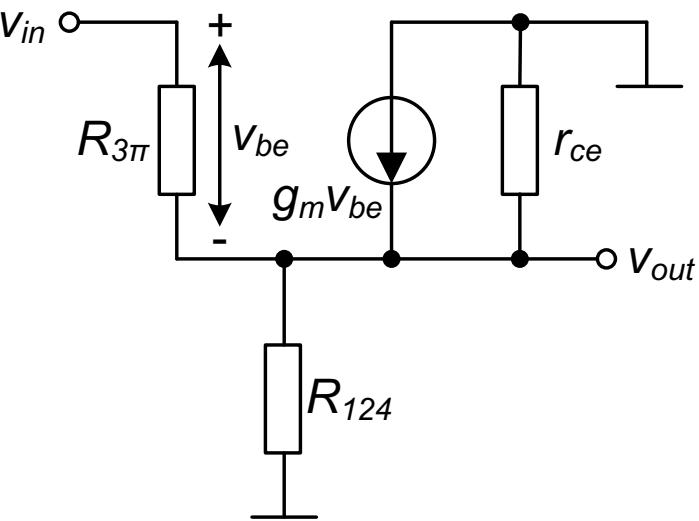
$$\frac{v_{in} - v_{out}}{R_{3\pi}} + g_m(v_{in} - v_{out}) = \frac{v_{out}}{R_{124}}$$
