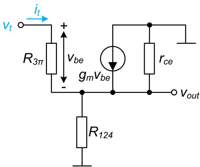
$$i_t = \frac{v_t - v_{out}}{R_{3\pi}} = \frac{v_t}{R_{3\pi}} \left( 1 - \frac{v_{out}}{v_t} \right) = \frac{v_t}{R_{3\pi}} (1 - A_v)$$
