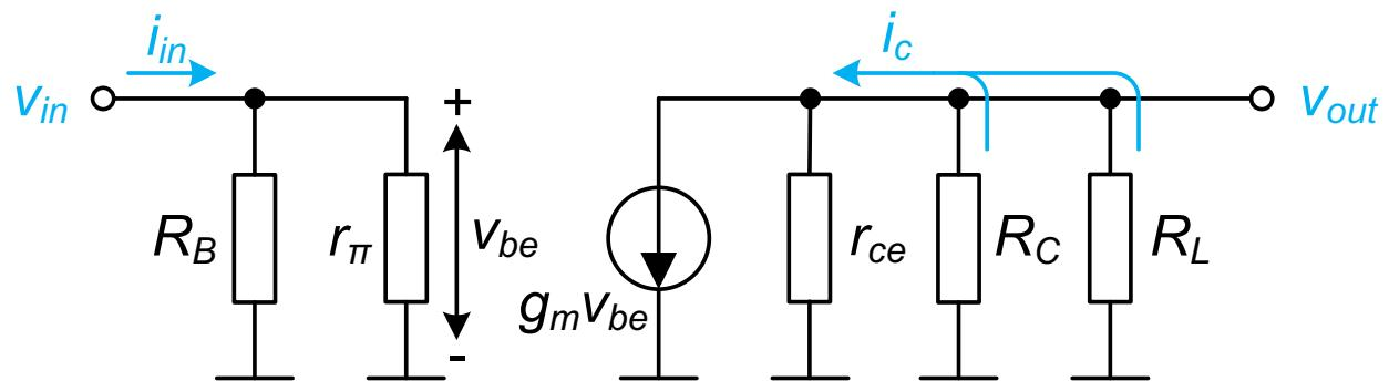
$$R_B = \frac{R_1 R_2}{R_1 + R_2} = 3.75 \text{ k}\Omega$$
