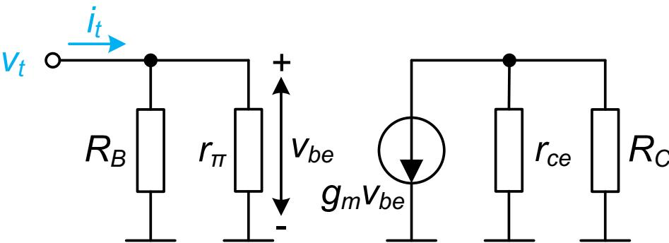
$$R_{in} = \frac{v_t}{i_t} = \frac{R_B r_\pi}{R_B + r_\pi} = 1.04 \text{ k}\Omega$$
